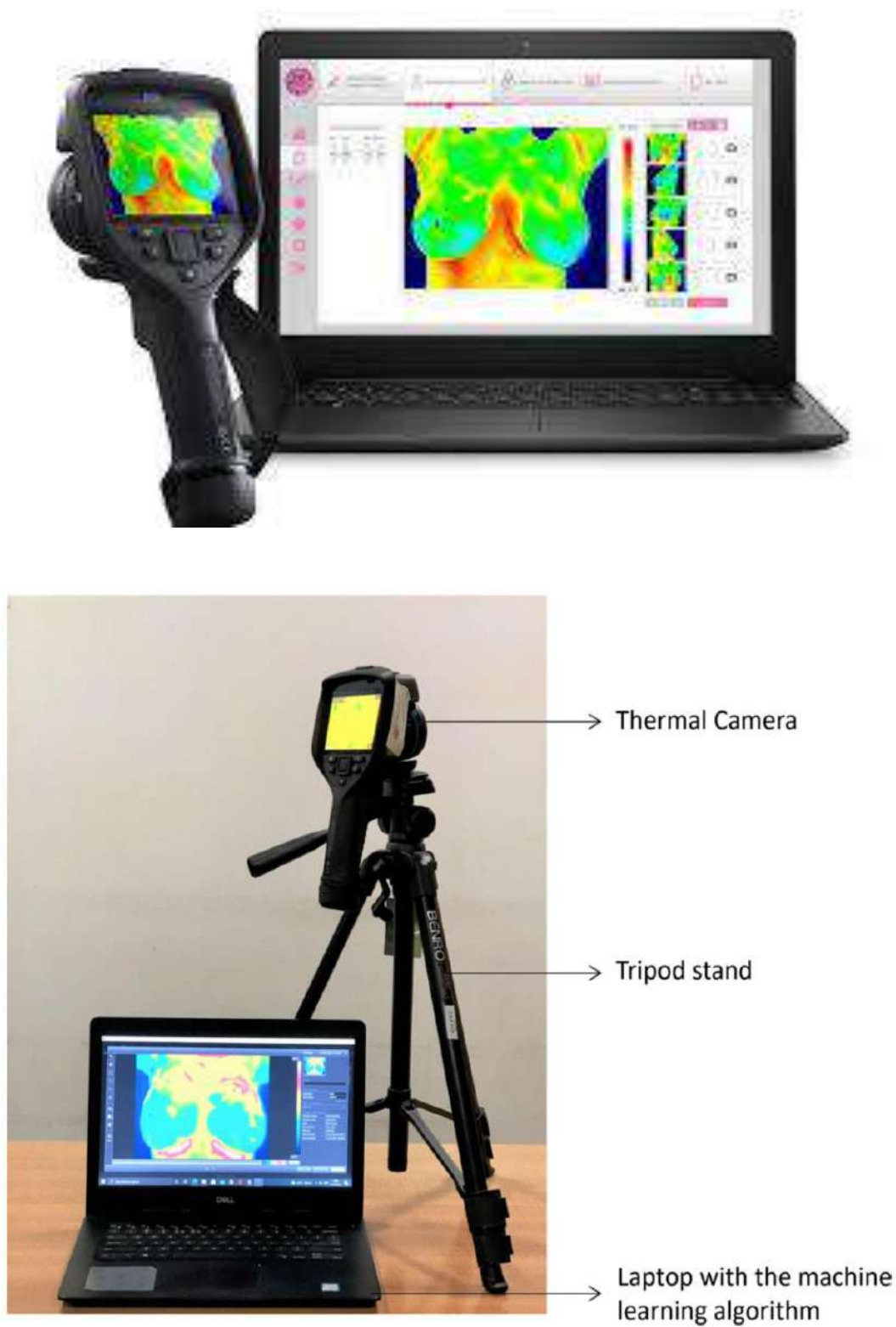
Figure 1: Test device – Thermalytix and its accessories
