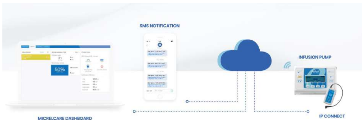
Figure 3: An innovative web-based care management tool designed to make patient monitoring an everyday practice. Healthcare providers can monitor the instant view of infusion status at 24 hours/day, receive clinical feedback for the patient, receive alerts in response to technical and clinical events and have instant access to the complete infusion history of patients.
